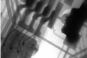
Image of a surface mounted IC permits inspection of the wires.
