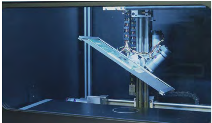
Glenbrook's Programmable Motion Control offers repeatable programs for automated inspection applications with precision within \pm 0.005" .
