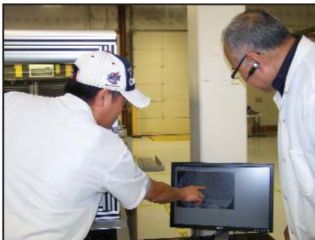
NCA operator Hoa Dao and VP of Program Management Cruz Alvarado inspect a memory card for voids and bridging.
